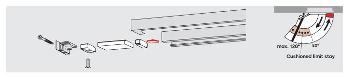
Accessories for the G-N, RF slide channel: Cushioned limit stay for retrofitting to the slide channel.
