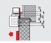
40 mm mounting backplate for G-SR For fixing the slide channels to the door frame where direct fixing is not possible.
