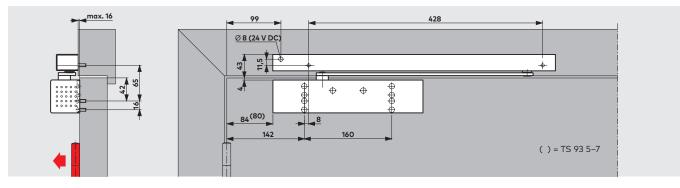
**TS 93 B** closer with G-EMF slide channel assembly, pull-side fixing Example: Anticlockwise-closing (ISO 6) door; mirrored arrangements apply to clockwise-closing (ISO 5) doors.
