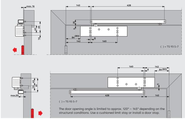
**TS 93 B** door closer with G-N slide channel assembly, door leaf fixing on the pull side and transom fixing on the push side. Examples: Anticlockwise-closing (ISO 6) door; mirrored arrangements apply to clockwise-closing (ISO 5) doors.
