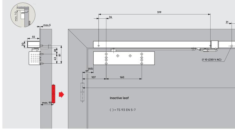
Door co-ordinator  ${\tt TS}~{\tt 93}~{\tt G}$  with integral smoke detector G-SR-EMR/BG, push side fixing
