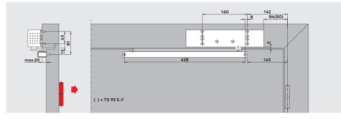
Transom fixing (overhead frame fixing) of the TS 93 B on the push side. Backcheck and delayed action non-operative with this fixing arrangement. The door opening angle is limited to approx. 120° to 145°, depending on the structural conditions. In order to prevent damage to the wall and door, a door stop should be installed to limit the maximum angle of door opening.
