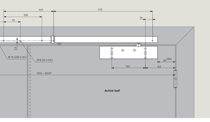
\* In the case of particularly large and heavy doors (over 2500 mm), we recommend that EM hold-open magnets be employed instead of the electro-mechanical hold-open unit.
