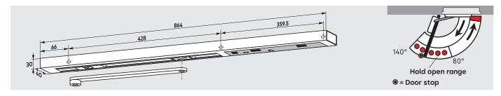
The **G-EMR** slide channel assembly enables fire and smoke doors to be held open securely at precisely the angle required, and monitored and controlled completely independently of other systems. The hold-open point can be adjusted to opening angles between approx. 80° and 140°.
