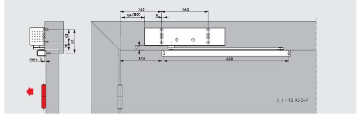
Transom fixing (overhead frame fixing) of the TS 93 G on the pull side.
