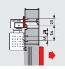
**40 mm mounting backplate for G-N, EMF, EMR** For fixing the slide channel to the door frame where direct fixing is not possible.
