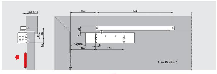
Door leaf fixing (standard arrangement) of the TS 93 B on the pull side.
