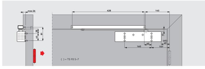
Door leaf fixing (standard installation) of the TS 93 G on the push side.
