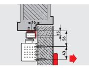
**Angle bracket for G-N** For push-side fixing of the slide channel to door frames with a deep reveal.
