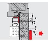
**Angle bracket for G-EMF** For push-side fixing of the slide channel to door frames with a deep reveal.
