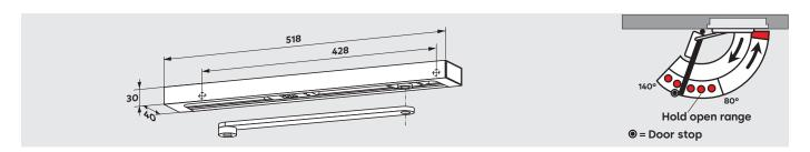
The **G-EMF** slide channel assembly enables the door to be held open securely at a preselected position without fall-back. The hold-open point can be adjusted within an opening angle of approx. 80° and 140°.
