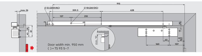
TS 93 G door closer with G-EMR slide channel assembly, push-side fixing
