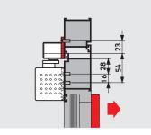
40 mm mounting backplate for G-SR/BG For fixing the slide channels to the door frame where direct fixing is not
