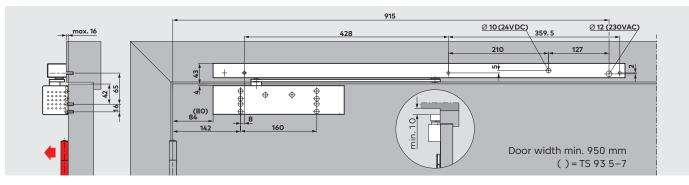
**TS 93 B** closer with G-EMR slide channel assembly, pull-side fixing Example: Anticlockwise-closing (ISO 6) door; mirrored arrangements apply to clockwise-closing (ISO 5) doors.
