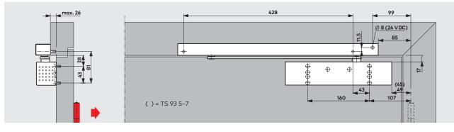
**TS 93 G** closer with G-EMF slide channel assembly, push-side fixing
