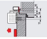
**30 mm mounting backplate for G-N** For fixing the slide channel to the door frame where direct fixing is not possible.
