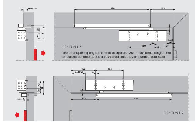
**TS 93 G** door closer with G-N slide channel assembly, door leaf fixing on the push side and transom fixing on the pull side. Examples: Anticlockwise-closing (ISO 6) door; mirrored arrangements apply to clockwise-closing (ISO 5) doors.
